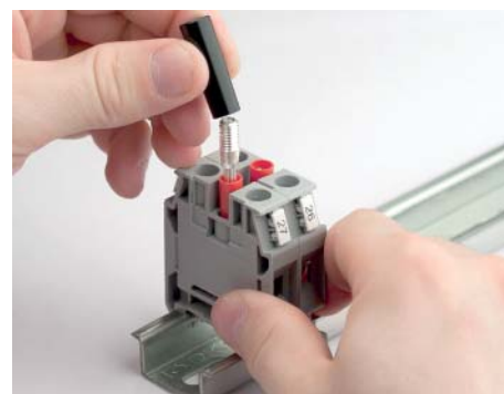
3. Secure a conductor in a probe with a clamp screw
